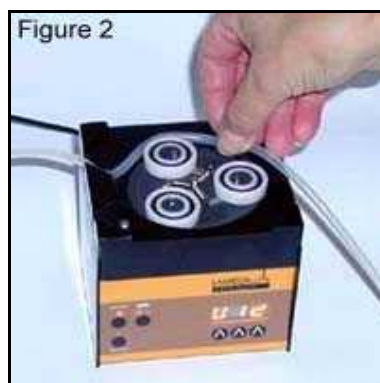
Fig. 2: Insertion of the tubing
