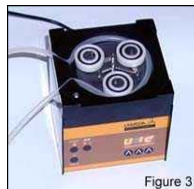
Fig. 3: Tubing in the pump head
