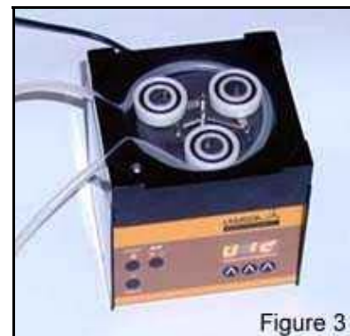
Fig. 3: Tubing in the pump head
