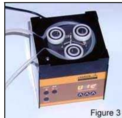
Fig. 3: Tubing in the pump head
